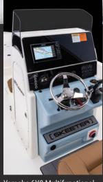
Yamaha 6Y8 Multifunctional gauges, elevator switch panel, EVA foam padding and a side access door.
